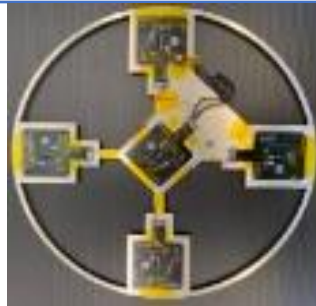
Wafer environment monitoring sensor system (wafer sense)
