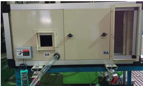
Integrated dedicated outdoor air handling system
