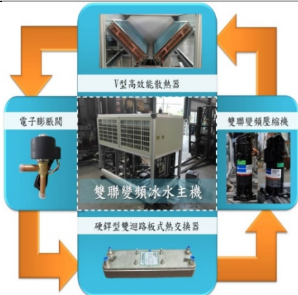
High IPLV and high COP double loop variable speed water chiller
