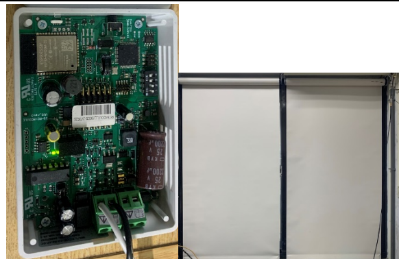
Smart linkage control of window shade and lighting for energy saving
